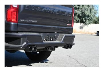
4) FINALLY, ADJUST TIPS TO DESIRED LOOK AND DEPTH THEN TIGHTEN. NOTE: THESE TIPS HAVE AN EXCEPTIONAL AMOUNT OF DEPTH ADJUSTMENT
